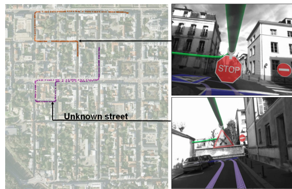
Figure 1: (a) Top view of the coarse 3D city model used in our experiments. (b) The final database superimposed on the satellite image. It comes from two georeferenced SfM point clouds. Their drift has been corrected with the process described in §2.
